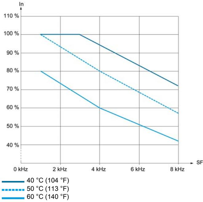
机架尺寸 7B — 380...480 V - 315 kW
